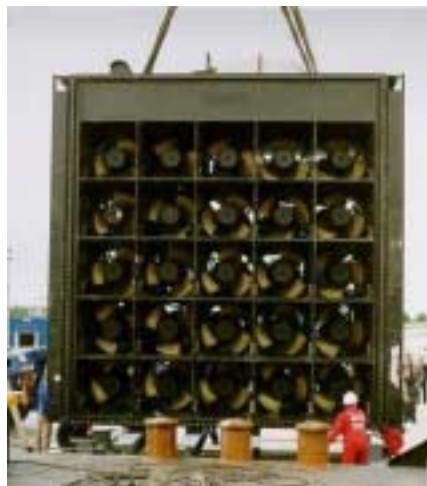
Figure 2-6 HYDROMATRIX™ grid of submersible turbines
