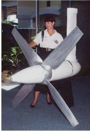
Figure 2-19 Prototype current turbine from NTU ( ee.ntu.edu.au/ntcer/projects/tidalpower/main.html )
