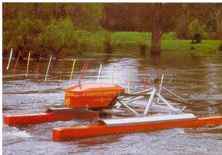
Figure 2-17 Tyson turbine, installed in the Murray River (members.ozemail.com/~tysonsturbine)
