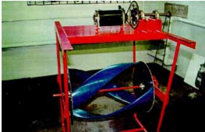
Figure 2-18 Helical turbine (picture from GCK Technology information pack)
