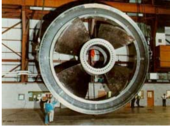
Figure 2-5 Straflo turbine from Annapolis (SULZER Technical Review, 1987)
